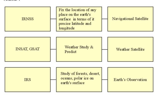
IRNSS: Fix the location of any place on the earth's surface in terms of it precise latitude and longitude: Navigational Satellite.
